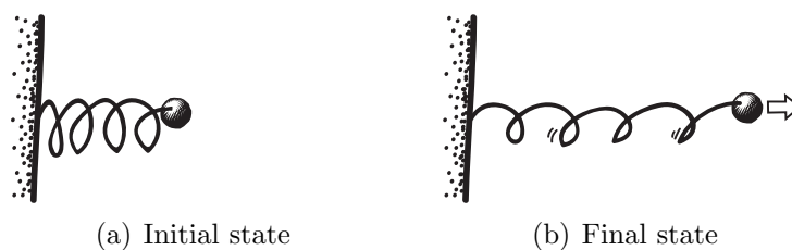
Figure 1. (a) A harmonic oscillator initially compressed out of equilibrium with zero momentum. (b) A final state for which the system has non-zero momentum.
